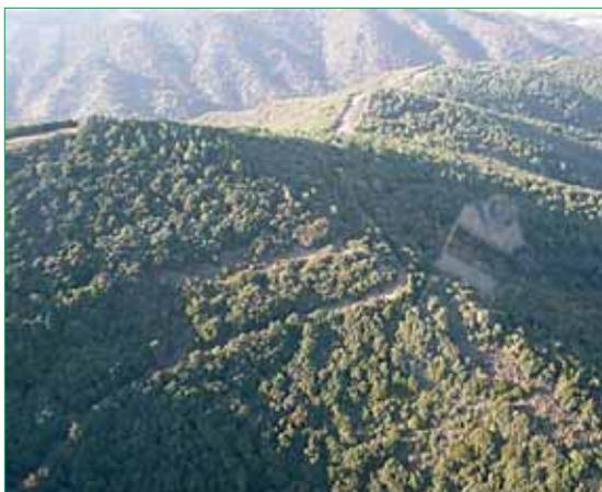
**Figure 132. Prades mountains.** Secondary track parallel to the ridge line and strip of low fuel load along the ridge line. Source: Bombers de la Generalitat de Catalunya.
