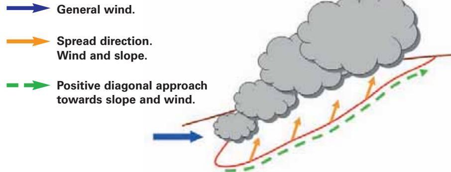
**Figure 130.** Positive diagonal approach towards slope and wind. Smoke and flames do not pass the advancing fire line. Source: Bombers de la Generalitat de Catalunya.
