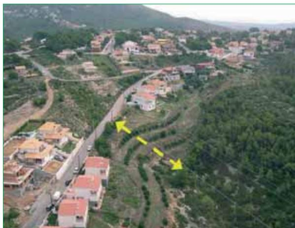
**Figure 16. Low-fuel-load strip protecting a residential area.** Source: Bombers de la Generalitat de Catalunya.
