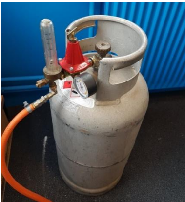
Illustration 3: The propane gas tank with a flow meter
