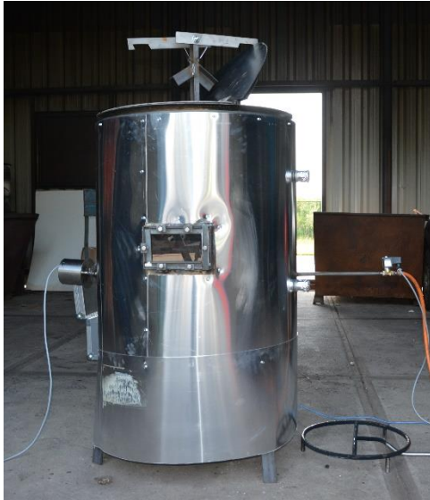
Illustration 2: Desktop flashover vessel with the burner in the right-hand bottom corner
