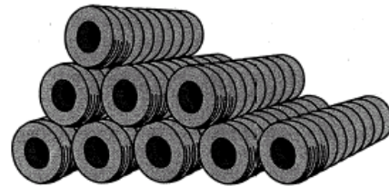
Figure 1-3(f) On-floor storage; on-tread, normally bundled; distance along tire hole not to exceed 25 ft (7.7 m).
