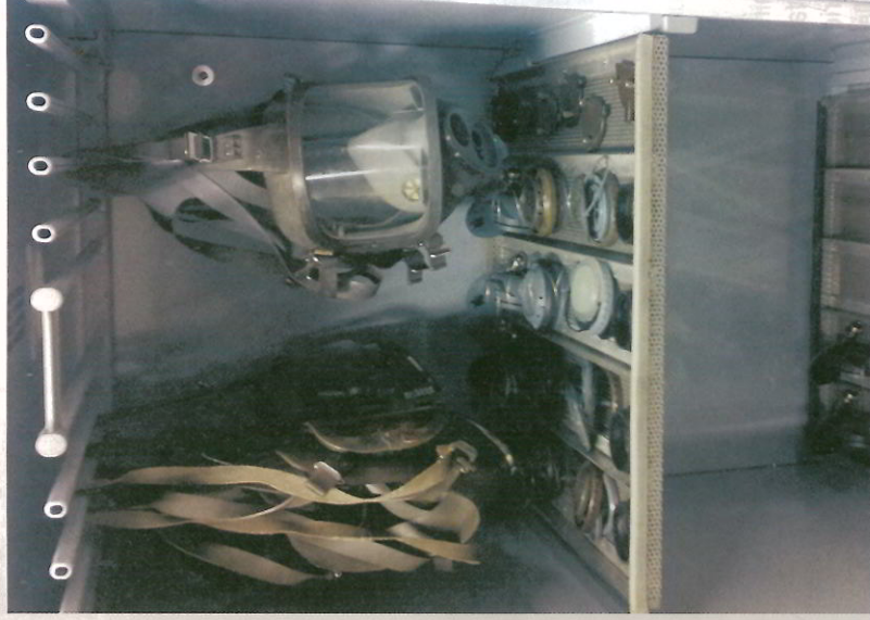
Breathing apparatus hanging in a drying cabinet.
